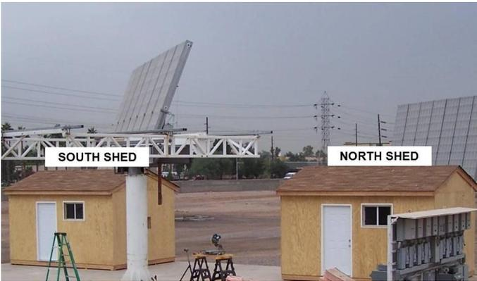
**Figure 2: EXPERIMENTAL SETUP OF SOUTH (NON BIOPCM) SHED AND NORTH (WITH BIOPCM) SHED**
